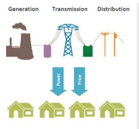
Consistent infrastructure for 100yrs Centralized generation One-way power flow Little to no control Simple fixed pricing Passive customers
